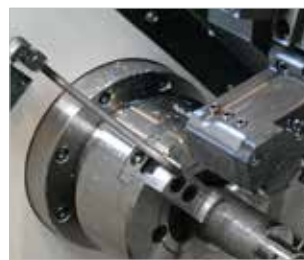
Chuck Air Blow (Upper Chuck)
