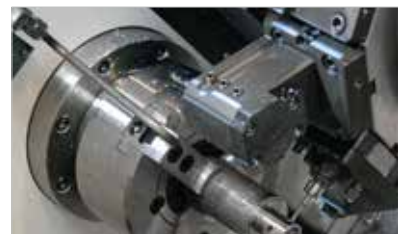
Chuck Air Blow (Upper Chuck)
