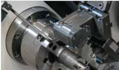
Chuck Air Blow (Upper Chuck)
